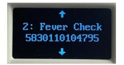
Pressing the lower key scrolls through the TRs of the different recorded chips.
